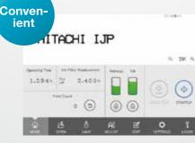
Icons on the screen indicate the ink and makeup amount of residue. They also indicate the proper time for cartridge replacement, which further improves usability.
